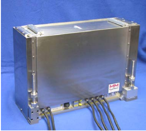
Figure 10: DC to AC converter ACC04
